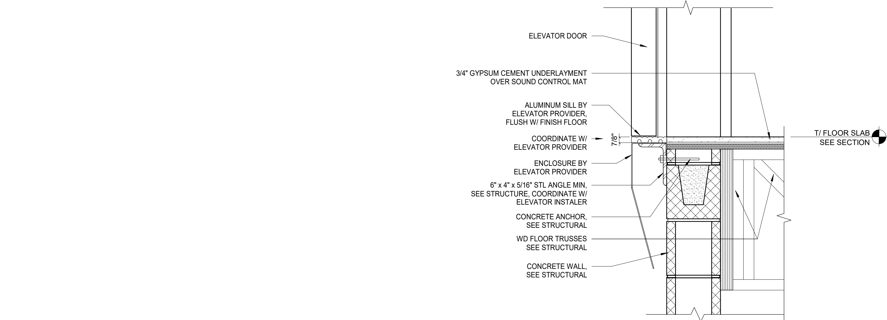
8 DETAIL ELEVATOR DOOR SILL - UPPER LEVELS 1 1/2" = 1'-0" REF: 6 / A602
